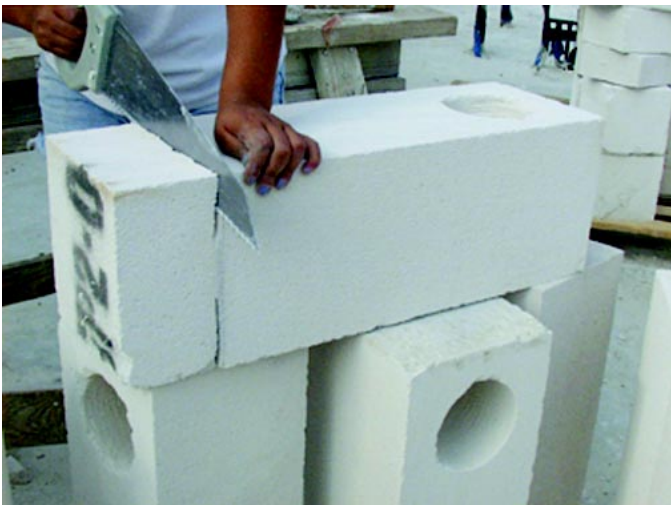
Aerated Concrete is sawed like lumber
