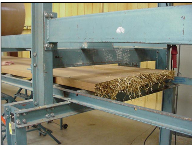
Wheat board assembly line at Affordable Building Systems in North Texas
