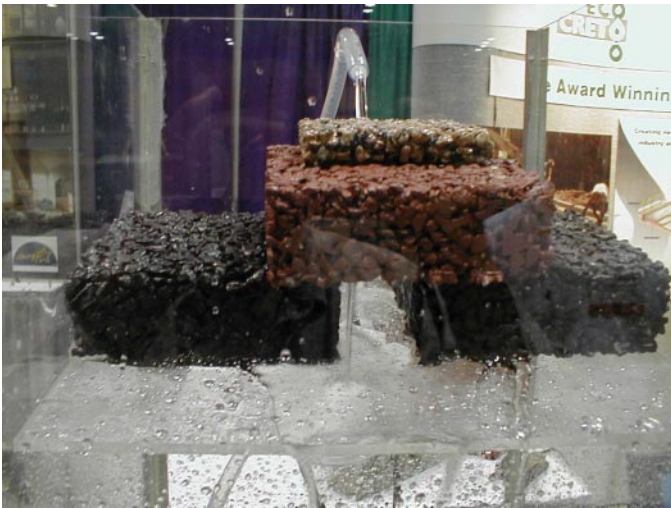
Water runs quickly through porous concrete
